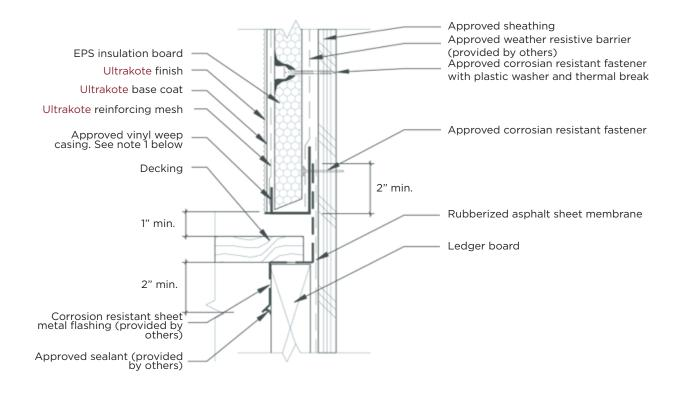
NOTE 1: Maintain 1/8" space between beveled insulation and weep casing bead. NOTE 2: All laps, spaces and corners in metal flashing shall be made permanently water tight.
